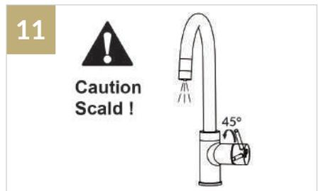
Press the button on the handle and turn the handle straight forward 45 degrees. The boiling water will come out of the faucet after 2-3 seconds. Caution Scald. See Fig 11
